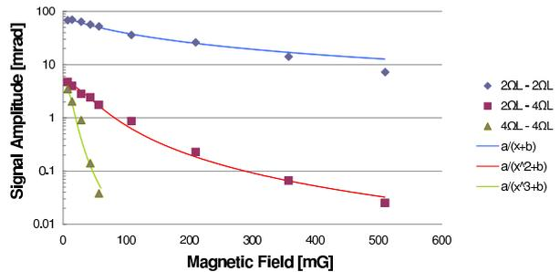
FIG. 3: Magnetic-field dependence of optical rotation amplitudes for quadrupole (blue diamonds), hexadecapole pumped with light modulated at  $2\Omega_L$  (maroon squares), and hexadecapole pumped at  $4\Omega_L$  (green triangles). The quadrupole and hexadecapole, pumped at  $2\Omega_L$  decrease much more slowly with magnetic field compared to hexadecapole pumped at  $4\Omega_L$ . The solid lines are fits by ad-hoc functions.
