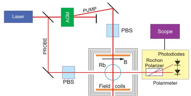
FIG. 1: Schematic of the experimental apparatus. The modulated pump light beam is used to polarize  $^{87}\text{Rb}$  atoms. The unmodulated probe beam is used to detect the evolution of the atomic polarization moments via induced optical rotation. AOM: acousto-optic modulator; PBS: polarizing beam splitters. See Methods.
